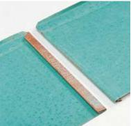
Prepare the tray ends according to the drawing and, using a 3 x 15 mm straight edge, fold ends 180° at 13 and 18 mm.
