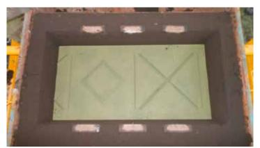
The main difficulty resided in defining the dimensions of the panels taking into consideration the deformation of the metal caused by stamping, and at the same time ensuring the system remains watertight. And subsequently in creating the stamping and bending die to test the quality of the product.
