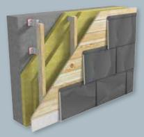
**Note:** ratio large to small = 2:1 panels To obtain an individual appearance over the whole surface area, vertical seams should not lie above one another (recommended minimum joint offset: 220 mm). Installation examples are available as a guide and can be downloaded (in PDF or DWG format) from www.prefa.com.
